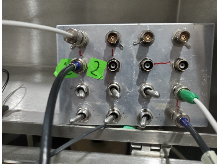
Figure 34. Switch box for four-point probe station. Box is used to convert from tri-ax cables to coax cables.
